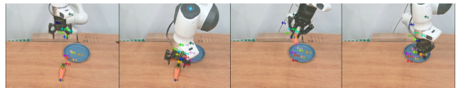
Fig. 3: Zero-Shot Sim-to-Real Transfer. A VC-1 backbone equipped with a GAP-pretrained spatial pooler applied to a real-world pick-and-place video [8]. The model successfully initializes and tracks the object and manipulator extremities without any real-world fine-tuning.
