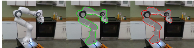
Fig. 1. We present a training-free approach for 6-DoF robot pose estimation that requires only a URDF model and joint configurations. Our method recovers the camera-to-robot transformation from a single real image without any robot-specific training. From left to right: input query image, ground-truth pose, and our estimated pose (rendered as URDF overlays).
